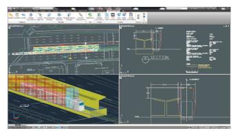
>> Accurately scale dimensions off the full scale report vehicle envelope clearance and tracking points relative to any structure envelopes.
